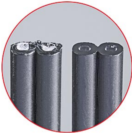
Differences in cut quality with a simple tool / with the cutting tool
